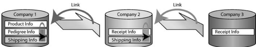
Fig. 4. A simple fragmented data approach to linking of pedigree data. Each company sends the next custodian a link to the pedigree data they hold for the product but retain the data themselves rather than embedding into a pedigree document.
